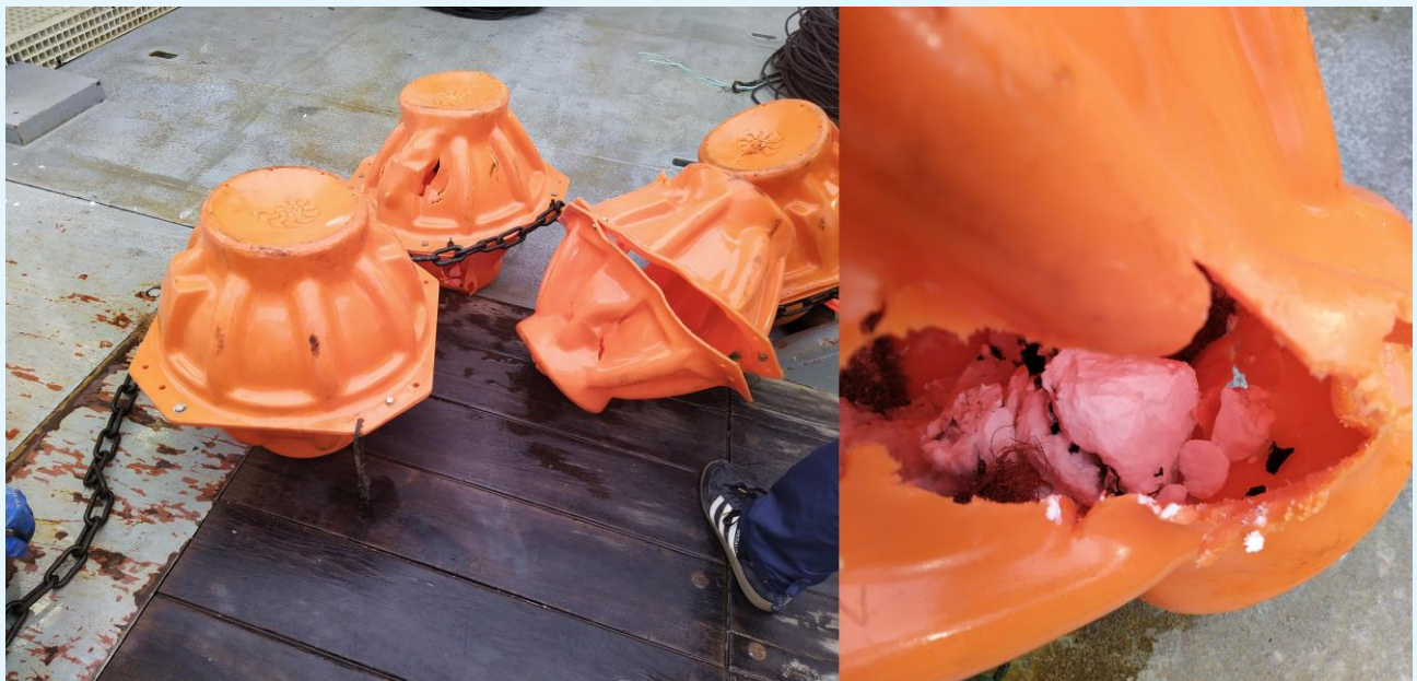
Figure 2. The deep glass flotation on mooring NWNM. Three glass buoys were destroyed leaving only the plastic cover. Probably they have imploded (the opposite of explode) turning the hard glass into a white powder. The flotation had been deployed at a depth of approximately 2400 meters, but they should be able to resist the pressure at up to 6000 meters.
